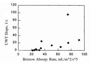
Figure 4. Correlation between the absorption rates measured with UWT and Bristow methods
