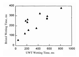
Figure 3. Correlation between the wetting times measured with the UWT and Bristow methods
