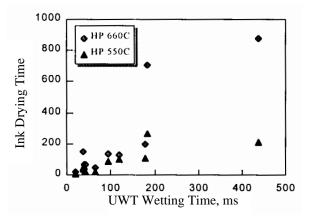
Figure 5. Ink drying index vs. wetting time measu red with the Ultrasonic Wettability Tester
