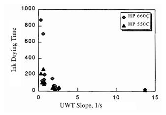
Figure 6. Ink drying index vs. absorption rate measured with the Ultrasonic Wettability Tester.
